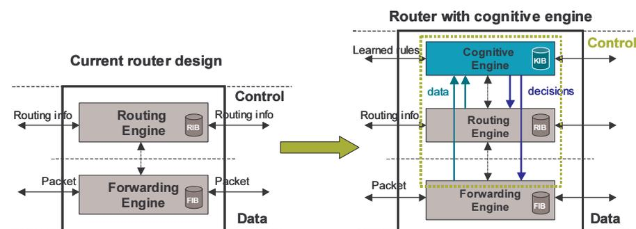
Fig.1: Cognitive engine and Cognitive router
